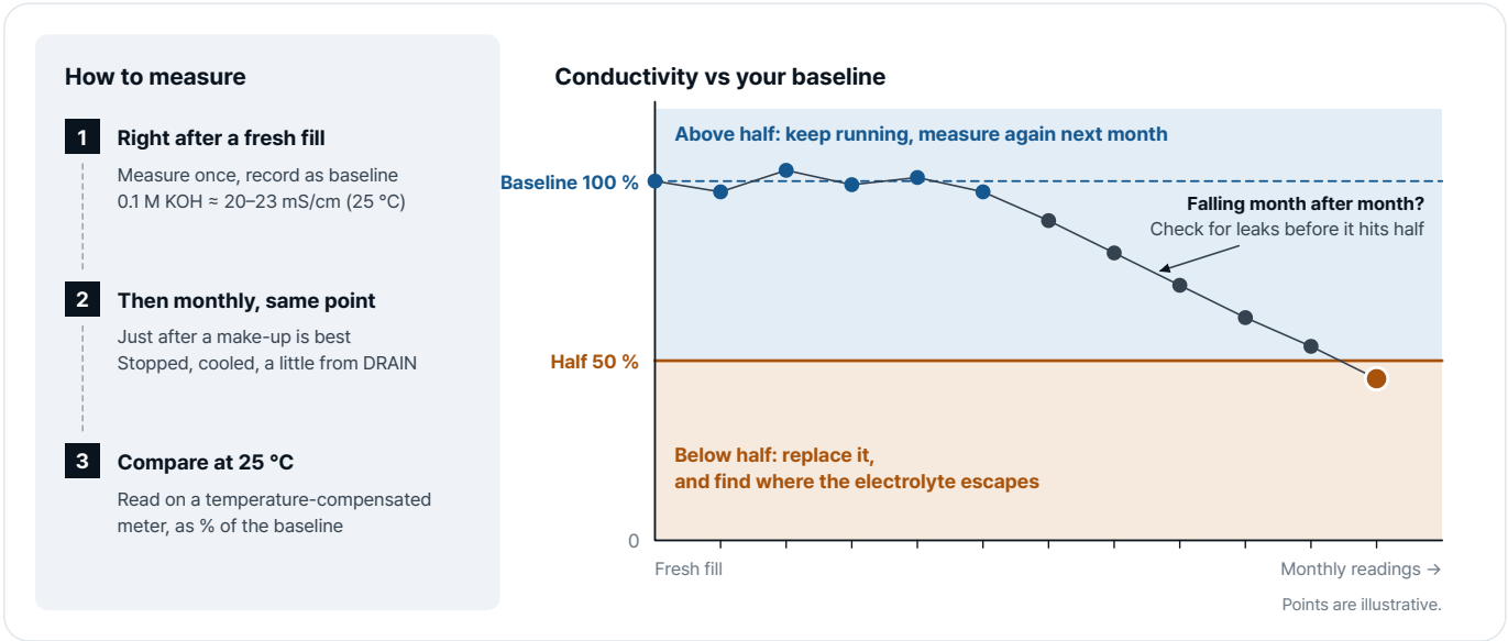
Figure 7-1 Deciding replacement from conductivity. Compare with your own baseline rather than the absolute reading. The points on the graph are illustrative.
